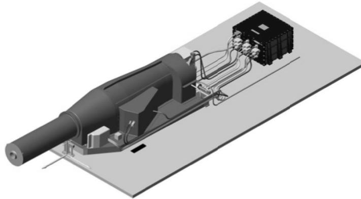
Figure 1. METIS Optical Unit (MOU) and MPPU accommodation on Solar Obiter panel
