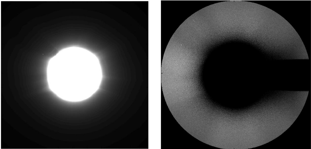
Figure 4 (left): A simulated un-occulted METIS FOV at 0.28 AU in the visible light (K+F) derived from a LASCO-C2 observation; palette threshold have been set to give some visibility to the corona features. (right): the simulated visible light image as acquired and digitized by the detector.
