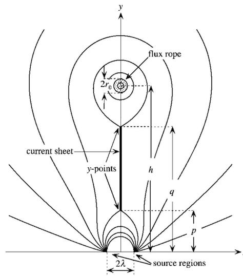
**Fig. 2.** Diagram of the Lin & Forbes (2000) CME/flux-rope configuration; this Figure can be compared with the observed configuration given in the middle top panel of Fig. 1.
